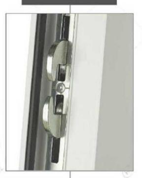
The Duplex Double Hook Lock has been designed by UK-based Ingenious' highly experienced and dynamic design team, providing a 6-point locking system instead of 3-hook for additional security. It comes with a dual follower to allow twin spindle function, which prevents unauthorised entry when the lock is in a latched position.
